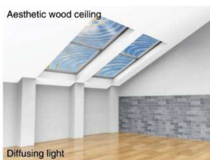
Figure 6: Comparing light diffusion through an aesthetic wood glazing with that through a standard glass ceiling. Adapted from Mi et al., 2020 under CC-BY licence
