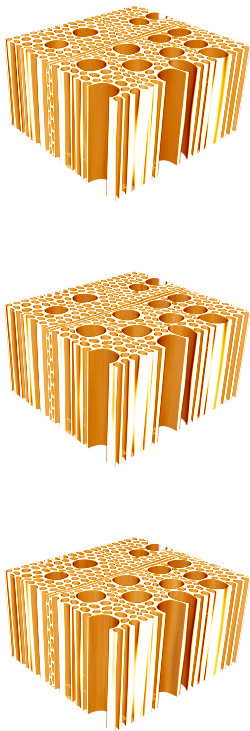
Fig. 12. A 3D birch microstructure of the size 550 \times 500 \times 300 generated by the original method (top), the surrogate model without transfer learning (middle) and the surrogate model with transfer learning (bottom).
